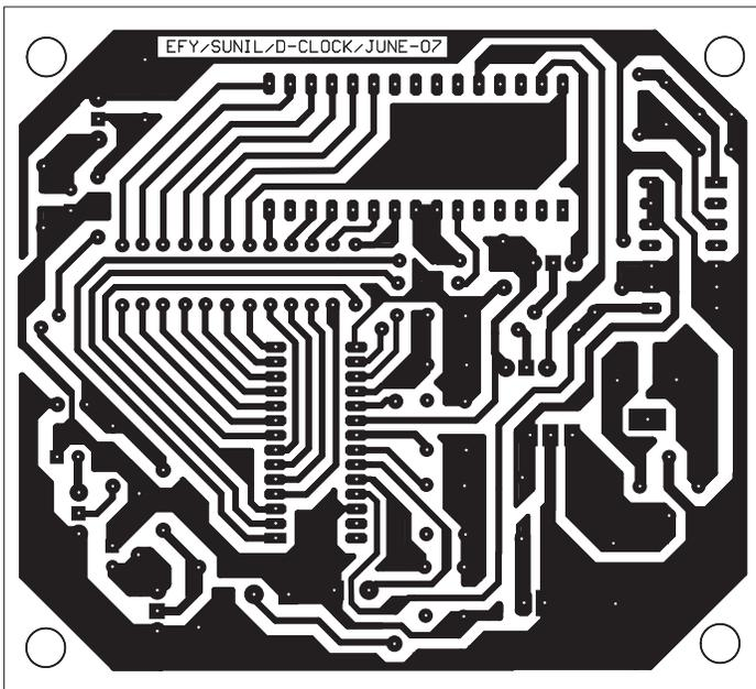
shows real time in hours and minutes. Pressing hour-set switch S4 makes the clock increment hours at 2Hz rate. Pressing minute-set switch S5 makes the clock increment minutes at 2Hz rate. Pressing both switches at the same time increments both
