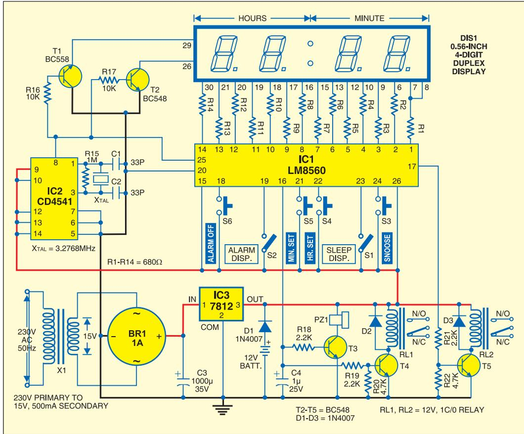
supply, all the lit segments begin to blink and the unit switches to a power-failure-detection mode. The power-failure-detection display is cancelled by activating Hours set S4 or Min set S5.
